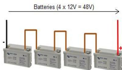
**Step 2:** Check polarity of the battery bank and identify the positive “+” terminal and negative “-” side.
