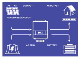
The photovoltaic production allows to supply the load and to charge the batteries. The grid supplies the additional needs to charge the batteries.
