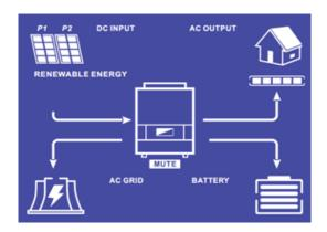
The photovoltaic production allows to supply the load, to charge the batteries and to feed-in the surplus of energy to the grid.
