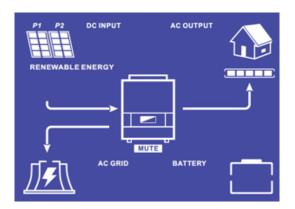
he « BATTERY » icon is flashing, the batteries are disconnected from the IMEON.
