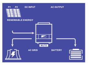
The photovoltaic production allows to charge the batteries and to feed-in the surplus of energy to the grid.
