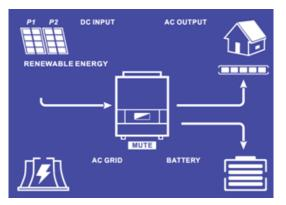
The « AC GRID » icon is flashing, the grid is disconnected from IMEON.
