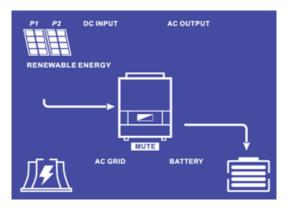
The « AC GRID » icon is flashing, the grid is disconnected from the IMEON.
