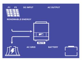
The « BATTERY» icon is flashing, the batteries are disconnected from IMEON.
