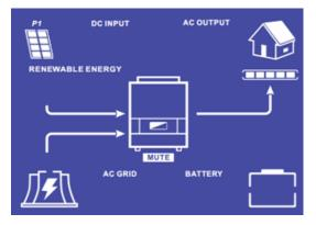
The « BATTERY » icon is flashing, the batteries are disconnected from the IMEON.
