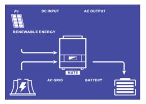
The photovoltaic production allows to charge the batteries. The grid supplies the additional needs to charge the batteries.
