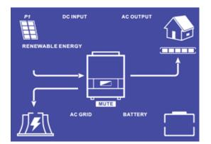
The « BATTERY » icon is flashing, the batteries are disconnected from the IMEON.
