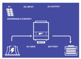
The « DC INPUT » icon is flashing, the photovoltaic panels are disconnected from IMEON.
