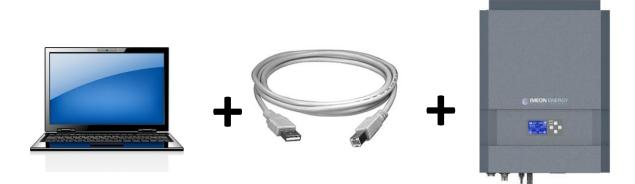
Connect the USB A /USB B cable between the PC and the inverter
