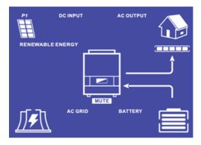
The « AC GRID » icon is flashing, the grid is disconnected from the IMEON.
