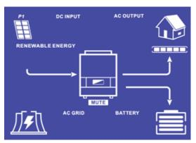
The « AC GRID » icon is flashing, the grid is disconnected from IMEON.
